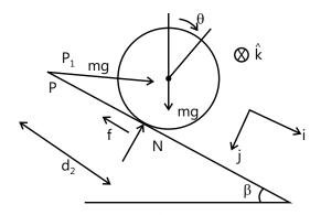
The gravitational force  $Mg = Mg \sin \beta \hat{j}$  acts at the center of mass. The vector from the point P to the center of mass is given by  $\vec{r}p.mg = d_p \hat{i} - R\hat{j}$ , so the torque due to the gravitational force about the point P is given by
