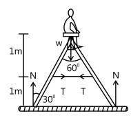
Next consider the equilibrium of the left leg of the ladder. Taking torque of the forces acting on it about the upper end.
