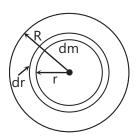
Considering, the solid sphere as a large group of hollow spheres whose radii range from 0 to R with a thickness of dr. Integrating moment of inertia of these dements gives the required value.
