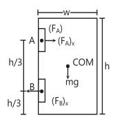
Given, hinge A is screwed while B is not, So, the upward component of force by hinge B is absent.
