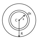
**Sol:** The disc can be thought of made-up of elementary rings of infinitesimal thickness. The torque about the center of disk due to friction force on each ring will be different from the other rings in the disc as the radii of rings are different, varying from 0 to R. So use the method of integration to find the torque on the entire disc.
