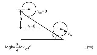
The magnitude of the velocity of the center of mass of the cylinder when it reaches the bottom of the incline
