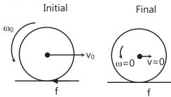
Frictional forces acts to reduce the velocity of bottom most point.
