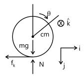
At t=0, when the ball is released  $v_{cm,i}=v_0$  towards right and  $\omega_i=0$ , so the ball slips towards right on the surface and hence the frictional force on the ball, will be towards left.
