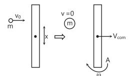
$$v_A = V_{com} - \frac{\omega L}{2}$$
