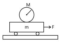
**Sol:** As the plank moves forward, the sphere, due to its inertia, has a tendency to slip backwards relative to the plank. So the force of friction acts on the sphere in the forward direction. For maximum force F, the friction will
