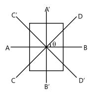
$$I_{ZZ} = I_{AB} + I_{A'B'} = I_{CD} + I_{C'D'} = 2I_{AB} = 2I_{CD}$$
