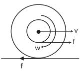
as  $\boldsymbol{\omega}$  is in clockwise direction, thread winds also friction acts leftwards to increase w.
