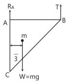
Center of mass of the triangular plate is at a distance of  $\frac{\ell}{3}$  from AC.
