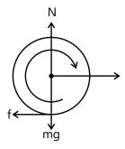
When the disc is projected it starts sliding and hence there is a relative motion between the points of contact. Therefore frictional force acts on the disc in the direction opposite to the motion.
