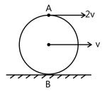
$$V_{\Lambda} = V + R\omega = 2V$$
