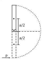
for minimum value of P, the angular velocity rod in the final position should be zero
