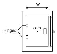
Suppose that m = 20.0 kg, h = 2.20 m, and W = 1.00 m and the bottom smooth hinge is not screwed into the door frame, find the forces acting on the door.
