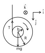
(a) The torque of tension in the cord about the center of mass of the Yo-Yo is in the clockwise direction. So as the Yo-Yo descends with linear acceleration  $a_{\text{cm}}$ , it rotates in the clockwise direction with angular acceleration  $\alpha$ .
