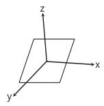
This theorem is applicable for planar bodies only and  $I_x$  and  $I_y$  should be about two perpendicular axes lying in plane.
