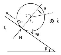
Then the only force exerting a torque about the center of mass is the friction force, and so we have  $f_sR = I_{cm}\alpha_z$
