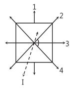
$I = I_1 + I_3$  (Perpendicular axes theorem)
