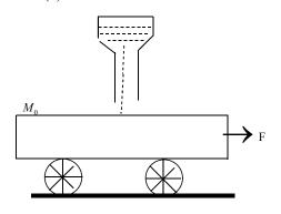
A) The velocity of the cart at time  $t(< t_0)$  is  $V = \frac{Ft}{M_0 + \mu t}$
