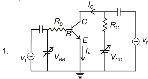
In the figure, given that  $V_{BB}$  supply can vary from 0 to 5.0 V,  $V_{CC} = 5V$ ,  $\beta_{dc} = 200$ ,  $R_B = 100 \text{ k}\Omega$ ,  $R_C = 1 \text{ k}\Omega$  and  $V_{BE} = 1.0\text{V}$ . The minimum base current and the input voltage at which the transistor will go to saturation, will be respectively:
