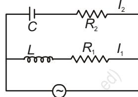
In the above circuit,  $C = \frac{\sqrt{3}}{2} \mu\text{F}$ ,  $R_2 = 20 \Omega$ ,
