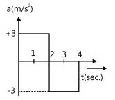
**Sol:** Area under the a-t graph in the given time interval is equal to the change in velocity of the particle in the given time interval. Thus v-t graph can be plotted if the initial velocity is known. Area under the v-t graph in the given time interval is equal to the displacement of the particle in the given time interval.
