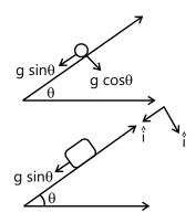
Acceleration of particle with respect to block
