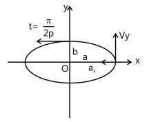
$\begin{aligned} t &= 0 \\ y &= 0 = v_x = a_y \\ x &= a \\ vy &= by \text{ and } \\ ax &= -ap^2 \end{aligned}$
