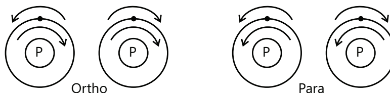
Figure 15.1: Spins for Ortho and Para Hydrogen
