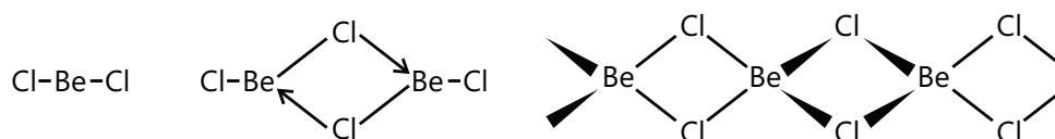
Figure 15.11: Beryllium chloride in solid state
