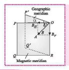
Relation between angle of  $dip(\delta)$  and components of earth's magnetic field.
