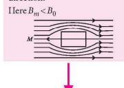
$\chi_m \to \text{Small},$ negative and temperature independent  $\chi_m \propto T_0$
